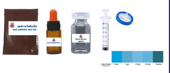
The prototype of soil salinity test kit including; Amber zip-lock bag, Clear vial 3 mL for AgNO<sub>3</sub> solution, Amber dropper bottle 5 mL, syringe 5 mL Filter and Color chart strip for estimating salt concentration.
